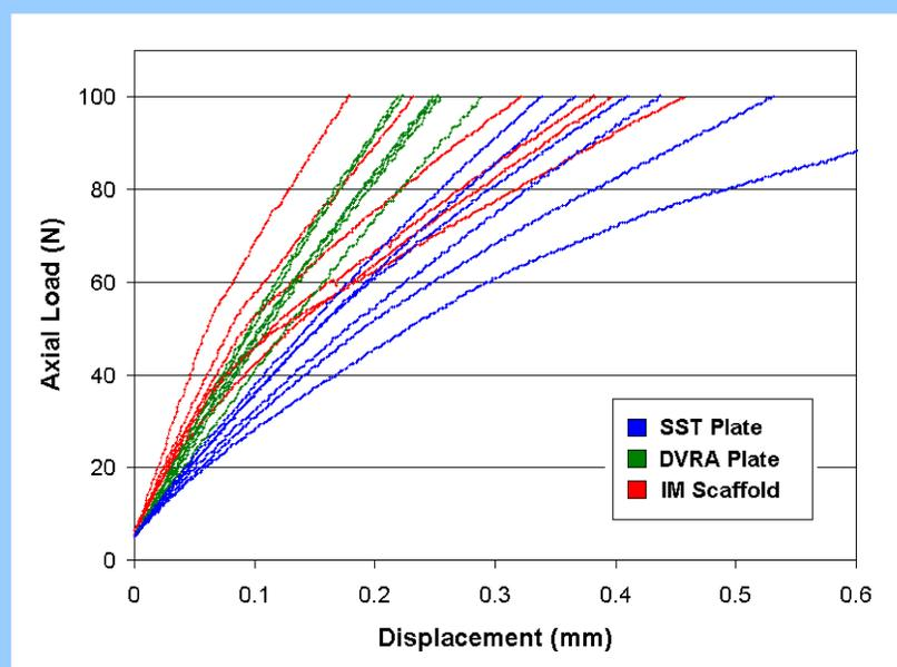
Fig. 5. Load-displacement curves at initial axial loading up to 100 N.
