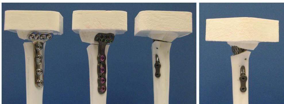
Fig. 3. (Left to Right) Non-locking T-plate, volar locking plate, and IM scaffold dorsal view; IM scaffold and wedge fracture lateral view.
