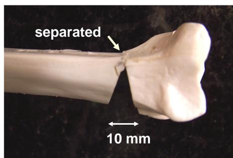
Fig. 2. Comminuted distal radius wedge fracture in foam bone model.
