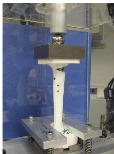
Fig. 4. Mechanical test system to apply axial and off-axis bending loading to specimens.
